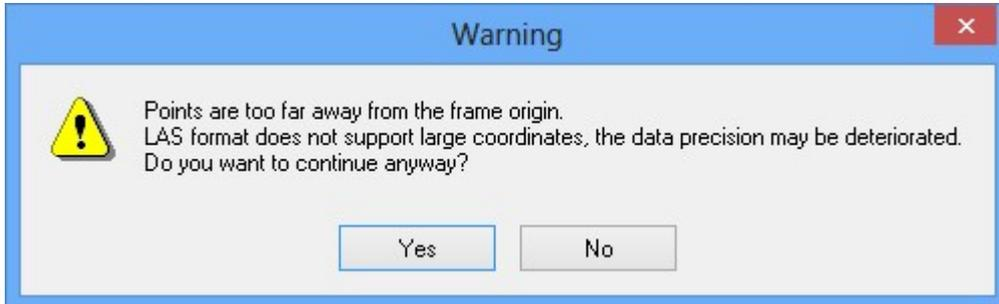
**Note:** An error message appears in case some layers are out of the **LAS** classification range. Some information may be lost because unsupported layers will be converted to "1 Unclassified", while compatible layers will be kept intact.
