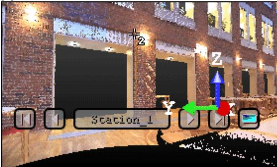
3. Pick another point on the screen so that the two points represent a horizontal segment in the 3D space. These two points define the orientation of a horizontal segment drawn on the final plane. The cursor becomes as shown in [C].
