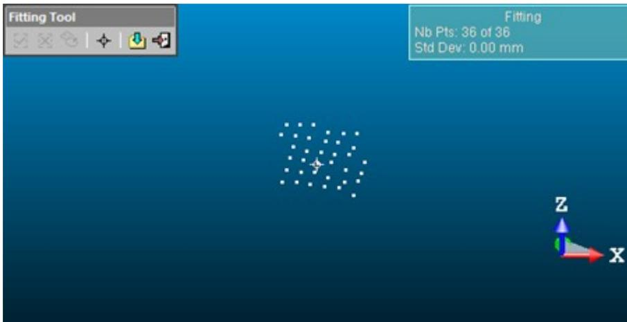
**Note:** An error dialog opens when **RealWorks** cannot find a **Point Target** close to the picked point.
