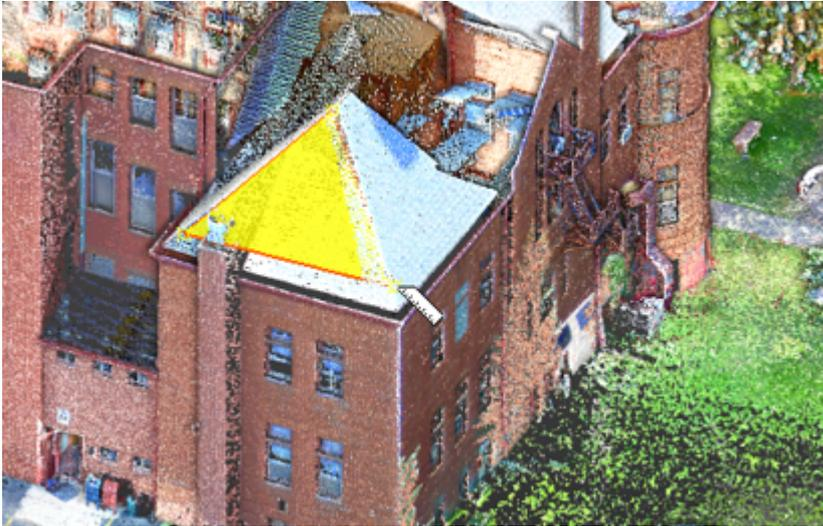
After picking the two first points, a temporary plane (of triangular shape) is displayed. As long as you move the cursor over a point of the displayed object, the temporary plane shape changes.
