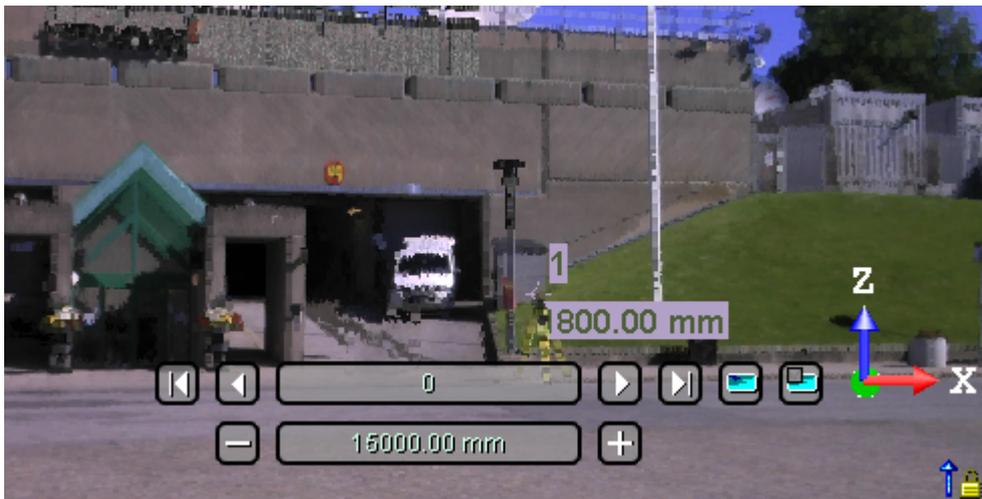
The scene is viewed from the first station viewpoint (the first in the **Project Tree**) with overlapped images in the background (see the upper illustration). You can use the **AutoSpin** feature in the **Preferences** to endlessly turn a scene around the station position. You can display (or hide) the position of the other stations as well as their label in the **3D**
