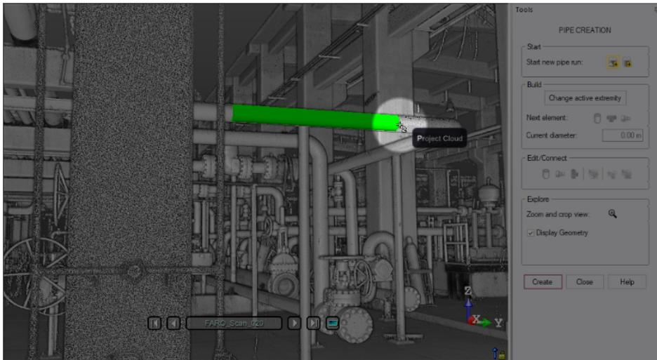
**Note:** The [Cloud Transparency](#) feature, which lets you visualize geometries without needing to hide the point cloud that is in front of, should be automatically enabled. If not, enable it.
