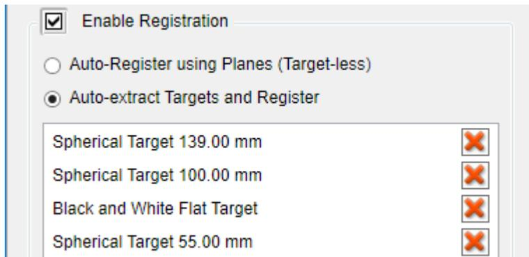
To remove a type of target to use, select it from the target list and press the **Remove** button at its right.
