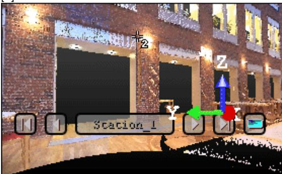
3. Pick another point on the screen. These two points will define the orientation of the first axis of the horizontal plane's frame. The cursor becomes as shown in [C] and the **Picking Parameters** toolbar appears in 3D constraint mode.
