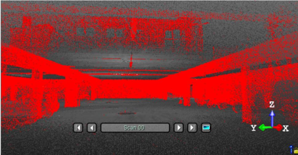
In the **3D View**, each picked point is used as seed to define a floor region, which is added to the previously extracted floor.
