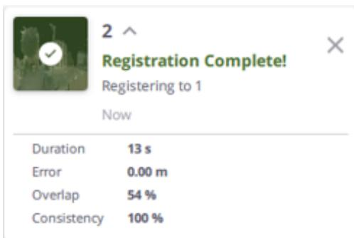
Each new station added to the project is automatically registered with the previous one, unless you choose a station from the **Register to** list. Stations that have been successfully registered per pair are put under the **Registration Set** (see [Edit & Register Registration Sets, page 41](#)).
