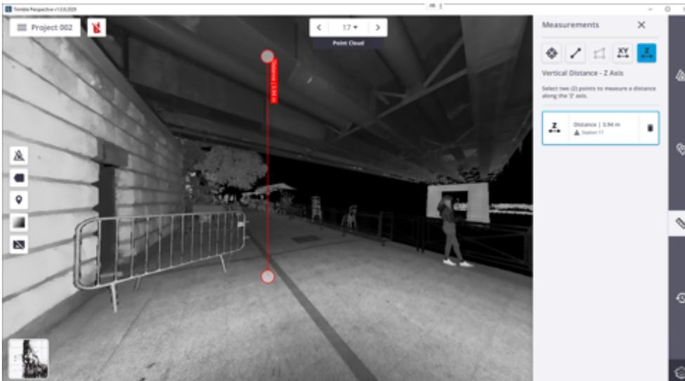
The measurement is performed between the first point and the projection of the second point along the Z axis.
