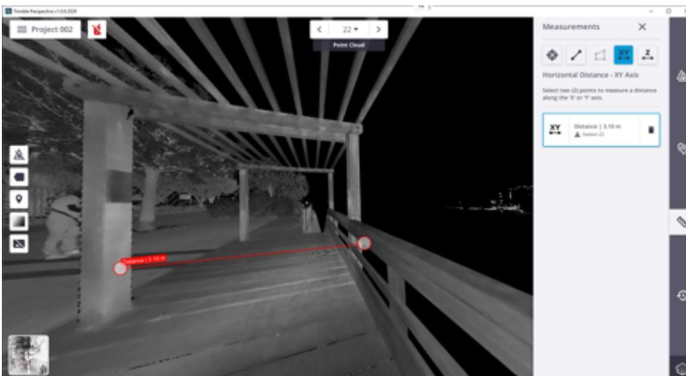
The measurement is performed between the first point and the projection of the second point in the XY plane.
